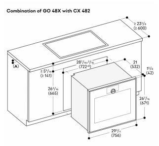
A: Min. worktop thickness  $^3/^4$  (20 mm) for surface-mounted installation,  $1^3/_{16}{}''$  (30 mm) for flush installation
