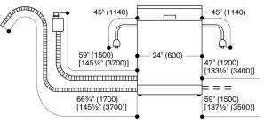
[] values with extension kit measurements in inches (mm)
