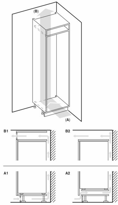
A: Air inlet  $\geq 200 \text{ cm}^2$ ; ventilation options A1 or A2
