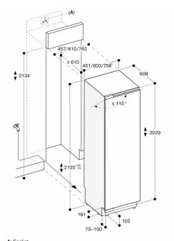
A: Socket Maximum door panel dimensions are based on a clearance of 3 mm
