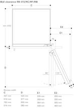
In the drawing, a unit front thickness of 19 mm and a Gaggenau unit handle of 49 mm were taken as a basis.
