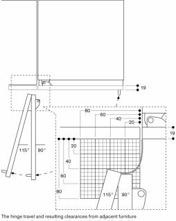
The hinge travel and resulting clearances from adjacent furniture units and handles can be found from the drawing while allowing for the thickness of the front panel. In the drawing, a furniture unit front panel thickness of 19 mm was assumed.
