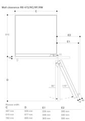
In the drawing, a unit front thickness of 19 mm and a Gagger unit handle of 49 mm were taken as a basis.
