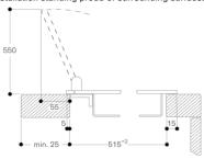
Installation with appliance cover/spacer batten; installation flush with surrounding surfaces
