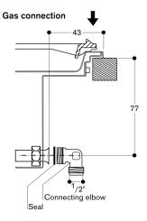
Minimum distance from the appliance cut-out to the side wall 150 mm.
