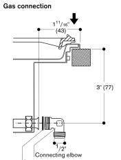
Minimum distance from the appliance cut-out to the side wall  $11^{13}/10^{11}$  (300 mm). measurements in inches (mm)
