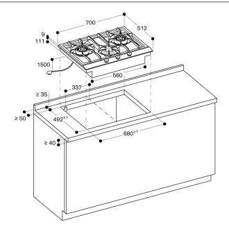
Minimum distance from the appliance cut-out to the side panel 300 mm.  $\,$ measurements in mm
