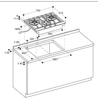
Minimum distance from the appliance cut-out to the side panel 300 mm. measurements in mm
