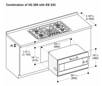
A: Min. worktop thickness 3/4" (20 mm) for surface-mounted installation
