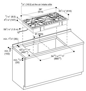
Minimum distance from the appliance cut-out to the side wall  $11^{1/3}$  (306 mm).
