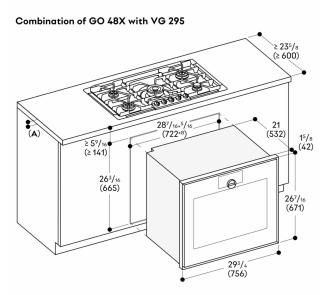
A: Min. worktop thickness 3/4" (20 mm) for surface mounted installation
