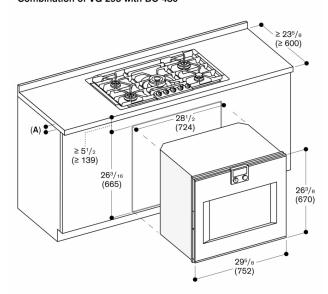
A: Min. worktop thickness  $^{3}/_{4}{}^{\shortparallel}$  (20 mm) for surface-mounted installation
