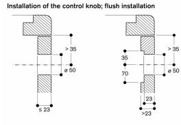
measurements in mm
