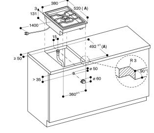
A: When installing with appliance cover, take the deeper cut-out into consideration (observe separate planning notes)
