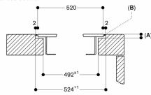
A:  $3.5^{-0.5}$  6.5 $^{+0.5}$ in combinations with frameless induction hobs B: Fill with silicone
