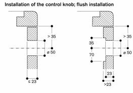
measurements in mm
