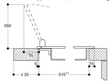
measurements in mm
