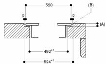
A:  $3.5^{-0.5}$  6.5 $^{+0.5}$ in combinations with frameless induction hobs B: Fill with silicone
