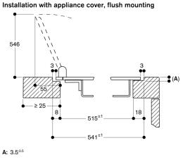
measurements in mm
