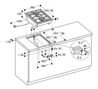
A: When installing with appliance cover, take the deeper cut-out into consideration (observe separate planning notes)
