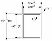
A: When installing with appliance cover, take the deeper cut-out into consideration (observe separate planning notes)
