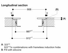
measurements in mm
