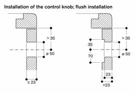
measurements in mm
