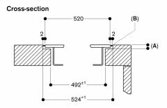
A:  $3.5^{\circ.5}$  6.5 $^{\circ.08}$ in combinations with frameless induction hobs B: Fill with silicone
