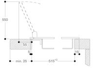
Installation with appliance cover/spacer batten; installation flush with surrounding surfaces
