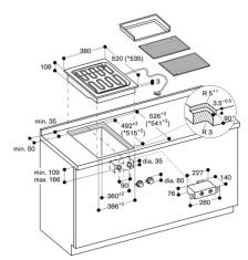
\* with appliance cover measurements in mm
