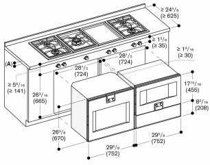
A: Min. worktop thickness  $^{3/4''}$  (20 mm) for surface-mounted installation,  $1^{3/16''}$  (30 mm) for flush installation
