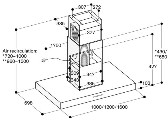
\* With air recirculation chimney AD 442 116, suitable for ceiling heights from 2.35 m to 2.60 m.
