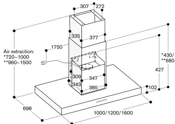
\* With air extraction chimney 442 016, suitable for ceiling heights from 2.35 m to 2.60 m.
